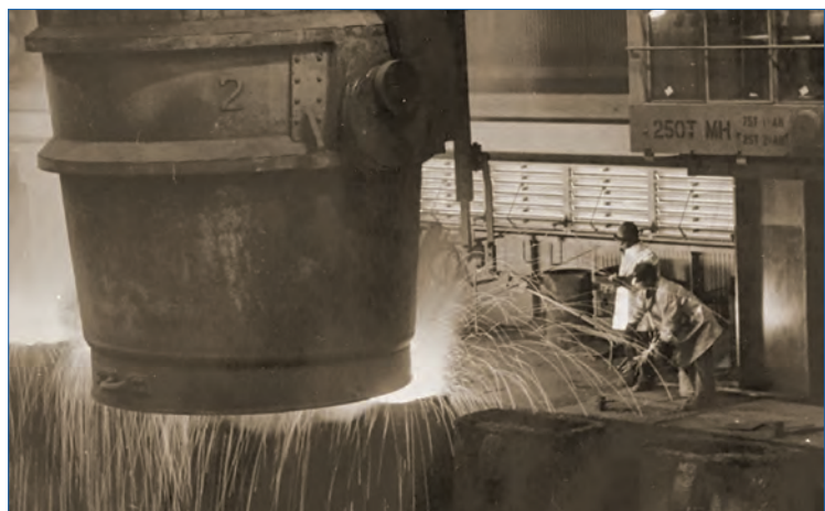
Pouring ingots at the then-new Basic Oxygen Process furnace—known as the "BOP Shop"—of U. S. Steel's Duquesne Works, 1964.
